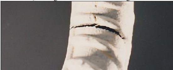
b) Low cycle fatigue longitudinal rebar (Photo: J Restrepo)
