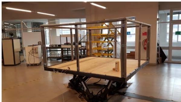
Figure 4. Shaking table testing system at University of Chile.
