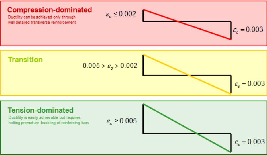
Fig. 9 Combined Flexure Axial Design Approach ACI318-08 Code.
