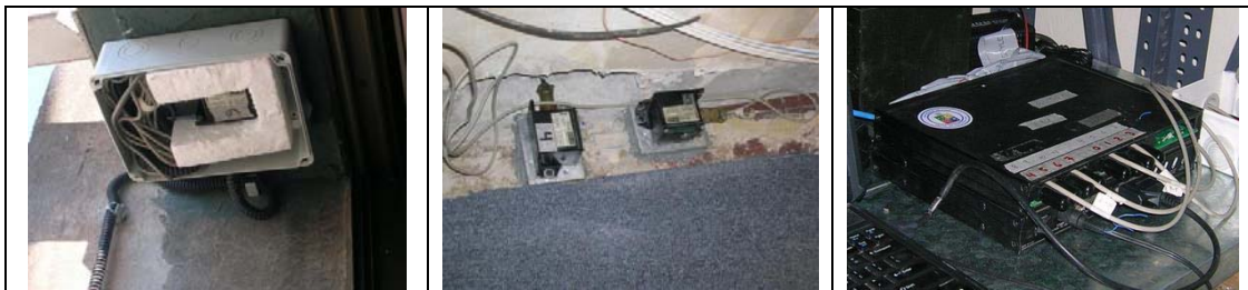
Figure 2. Accelerometers and acquisition system.
