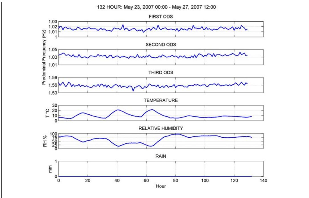
**Figure 6. Modal Parameter Variations with Temperature in a single 132 hour period.**
