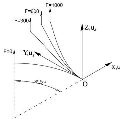
Figure 9: Initial geometry and some examples of the deformed configurations for the linear elastic case of the 45° cantilever bend.
