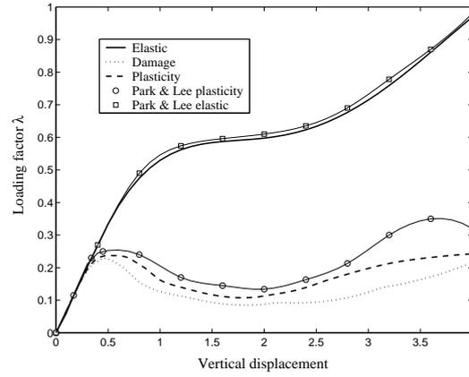
Figure 8: Loading factor-displacement curve of the vertical apex of the dome.
