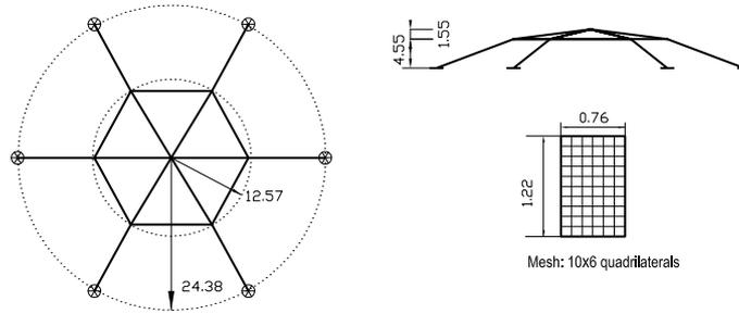
Figure 7: Framed dome and detail of the cross sectional mesh.
