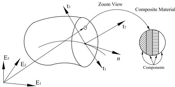
Figure 2: Cross section showing the composite associated to a material point on the current configuration.
