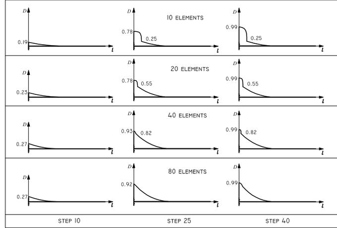
Figure 6: Evolution of the local cross sectional damage index: Strain localization. The symbols  $D$  and  $l$  are the damage index and the length of the beam, respectively.
