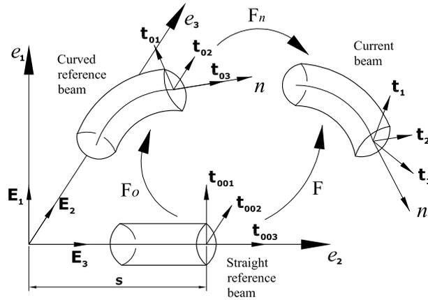
Figure 1: Configurational description of the beam.
