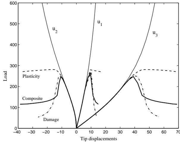
Figure 11: Different components of the tip displacement.
