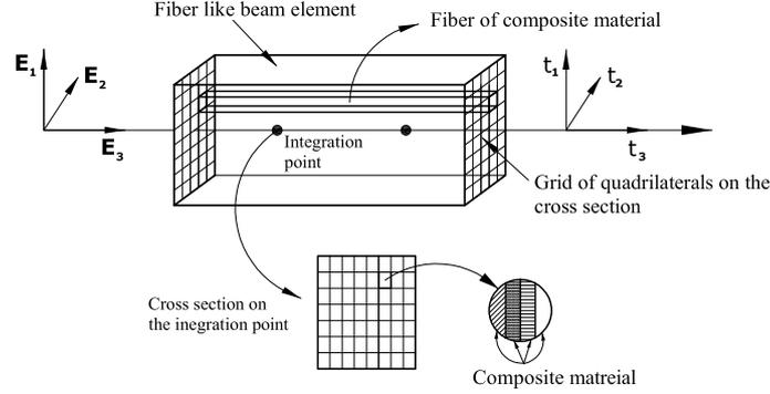
Figure 3: Discrete fiber like model of the beam element.
