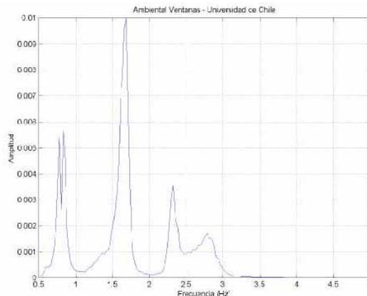
Fig 18 Power graph of the microvibrations registries
