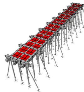
In addition calculated in manual form the rigidity of the deck 3 N° and N° 4 to reaffirm the obtained value of program SAP 2000. For the deck N° 3 gives a value of 29 ton/cm and for the deck N° 4 gives 22 ton/cm.
