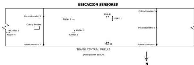
Fig. 11 Location of sensors in deck N°4
