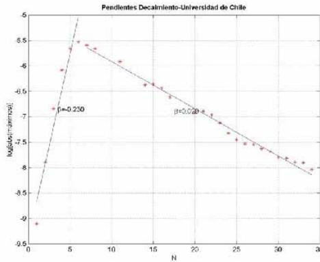
Fig.15 Obtaining of damping in base to the registries
