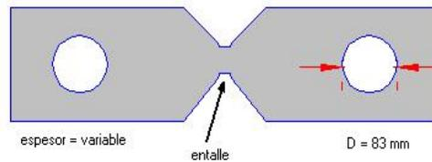
Fig. 8 Design of the final Fuse
