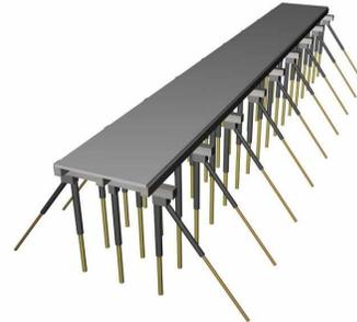
The steel structures are marks that are to the sides of the section. Alongside North they support to the asphalt pipes and their derivatives. Alongside South they support to the conveyor belts and the line of sulfuric acid.
